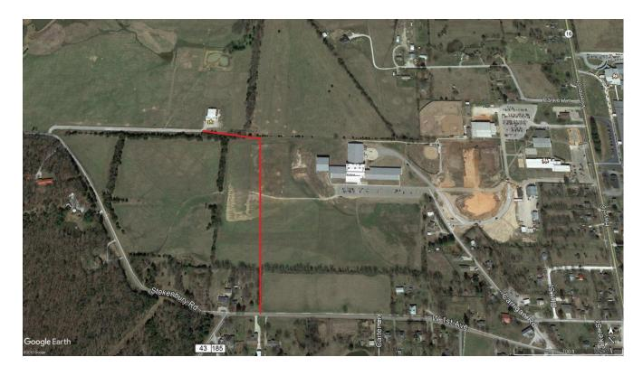
3. Plan to connect existing street stub on Braswell Rd to Hwy 16 with a 2-lane collector in order to provide another outlet from Stokenbury Farms subdivision and any future development in that area.
